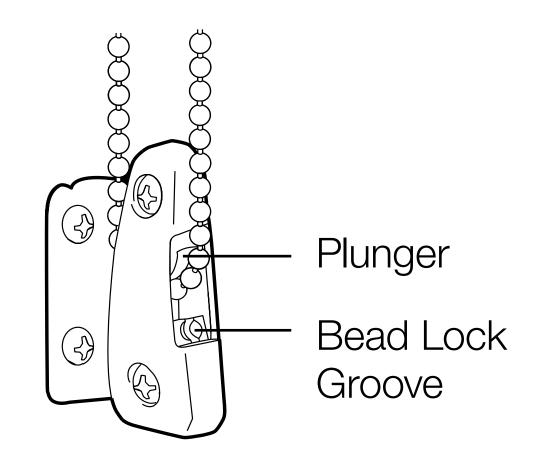
Pholding control loop, pull tension device down until loop is taut and plunger spring is fully contracted. Then move tension device up approximately <sup>1</sup>/<sub>8</sub>" to relieve stress on control loop. Do not twist or cross the loop.
